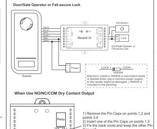
The power supply's voltage must be the same with lock's supply voltage, or else, the lock will not work properly or be damaged.
