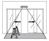
The door will open when a object put within the detection area.(as picture showed)
