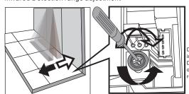
Detection range towards inside by clockwise rotation. Detection range towards outside by counterclockwise rotation
