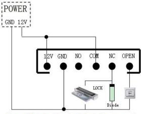
Remark: If let relay drive electric-lock, please connect a reverse diode with the lock's "+" and "-" poles.
