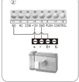
Attention! then electronically controlled lock must be transferred to 0 seconds delay, to prevent burning of electric locks.
