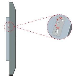
You can set the operation mode of Fail Safe or Fail Secure.
