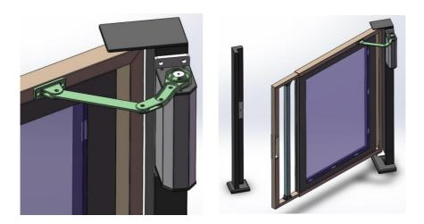
C. Install the main body of the door opener according to the size provided in 2.1.2 and 2.1.3.
