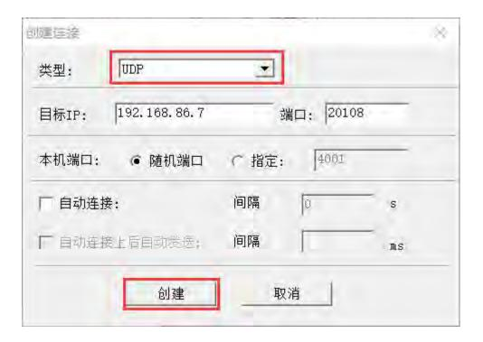
8. After pressing the "Connect" button, use 16 binary mode to send and receive instructions;
