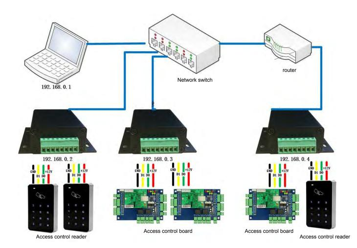
The network module uses UDP SERVER / CLIENT protocol or TCP SERVER / TCP CLIENT protocol, the specific protocol can be negotiated with the software developer;
