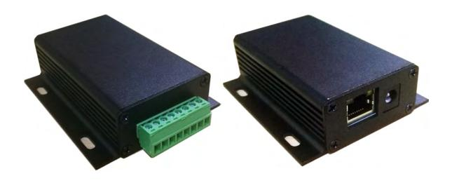
The converter needs a power supply of 9-24V 100mA (when using a 24V power supply, please
