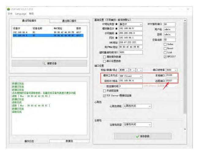
The receiving end should also be set to UDP CLIENT mode, and the destination IP should be set to the sending end address,
