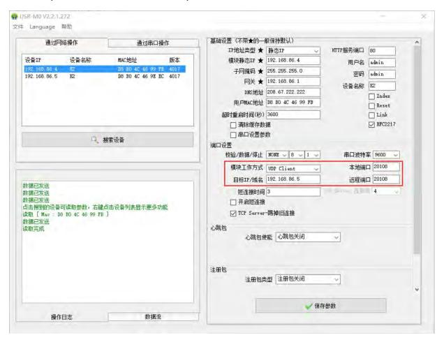
The sending end is set to UDP CLIENT mode, and the destination address is the IP address of the receiving end converter
